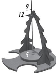
5.) Push in the wings diagonal into the slots of the perforated disc. All wings have to point at the same direction. The position of the wings decides the direction of rotation.
